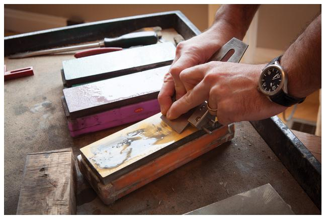
Rock 'n' roll. Use finger pressure to make the iron rock back and forth on the stone as you roll the honing guide up and down the stone.
