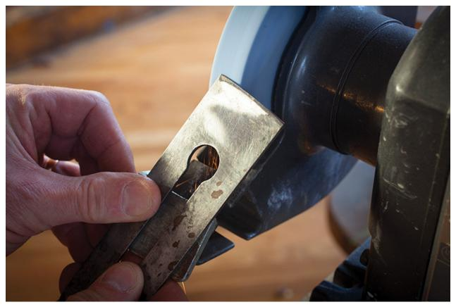
Wave bye-bye to straight edges. After establishing the bevel with short strokes, you can then work the entire bevel in a single stroke. The wrist motion is like waving goodbye.
