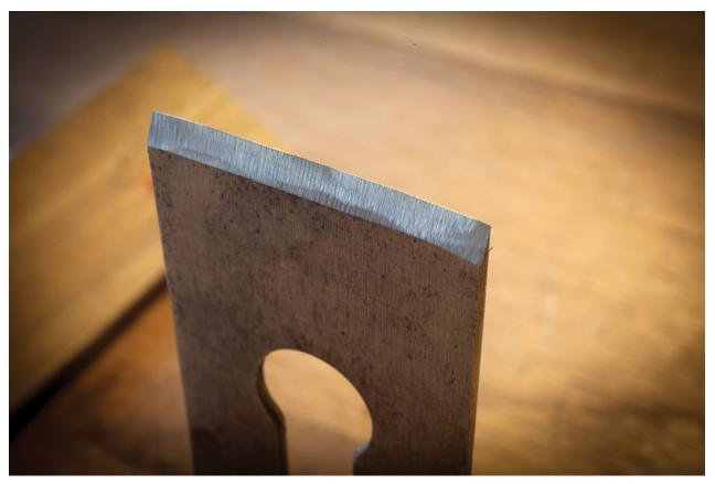
Tiny flat. This is when I switch from the grinder to stones. The flat is there, but it is barely visible.
