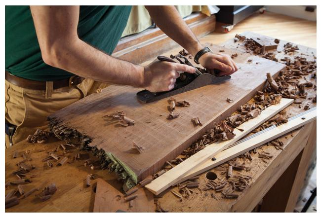
With a twist. When your board is in wind, plane diagonally across the two high spots to bring them down to the low spots. If you are removing twist from a big tabletop, you might have to plane locally at the two high corners first.
