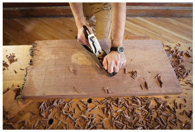
Skewed but straight. To reduce tearing, skew the tool in the direction the grain is running but push the tool straight across the board.
