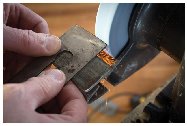
The right curve. Grind to the line on the back of your iron (above). When you are done, the flat on the edge should look like this (below).
