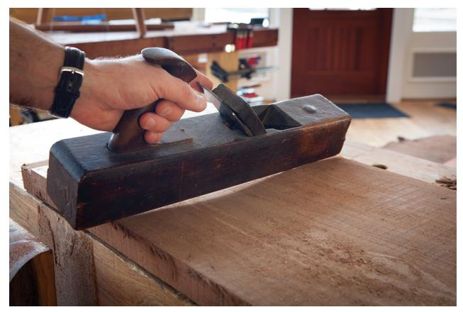
Conquer the cup. With cupped boards, traverse the high edges to bring them down to the valley between.
