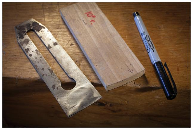
Around the bend. A wooden template of the desired curve is a handy thing to have next time you need to grind the iron – or for grinding your neighbor's fore plane.
