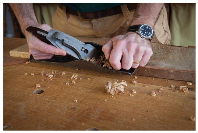
Stop spelching. A heavy bevel on the far edge will prevent spelching when you traverse a board. The bevel can be ripped away after you flatten the board.
