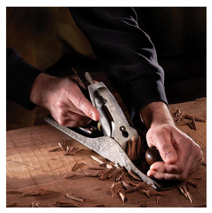
Flattening surfaces that are cupped, bowed or twisted had traditionally been the job of the fore plane, a tool that is used mostly by working across the grain of the wood. And sometime in the 20th century, the fore plane fell out of favor among woodworkers as the prices of electric jointers and planers dropped to the point where almost anyone could afford machinery.
