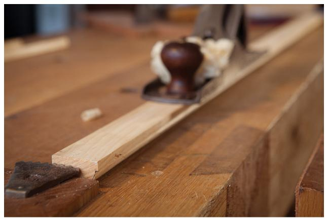
Remove bulk. A fore plane can quickly remove material that is interfering with a tight fit between your moulding and carcase.
