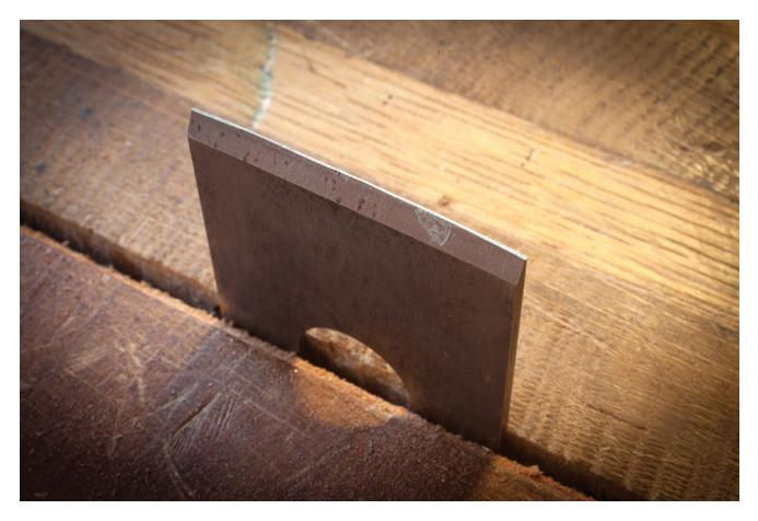
So set the grinder's tool rest so the blade is 90° to the wheel. Grind down to your line. You'll find this process goes quite rapidly with little pressure, so take it easy. It's unlikely, but if the edge heats up so much that you cannot touch it, cool the steel in a cup of water.
